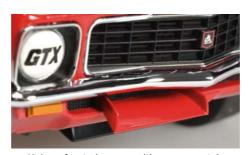
Unique front air scoop with woven metal mesh in behind it.
